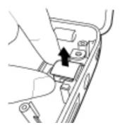
Figure 4-33 Removing DC in cable
